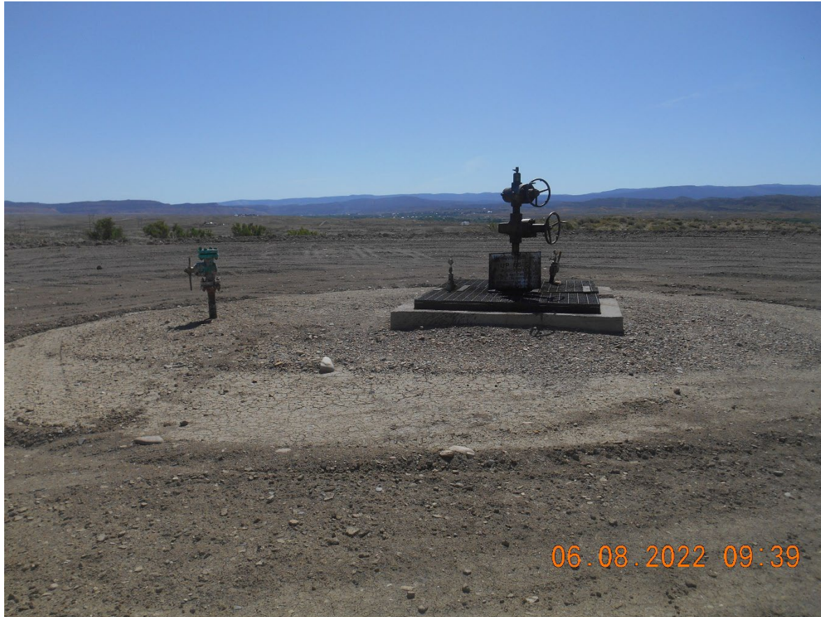
Injection wellhead. Temporarily abandoned.
