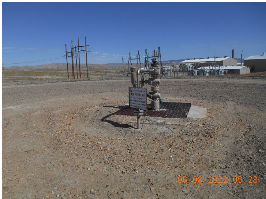
Injection wellhead.
