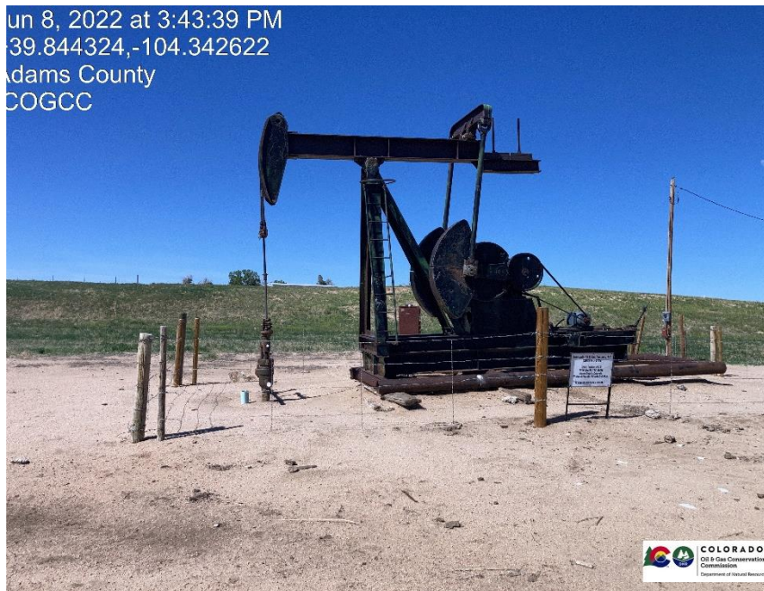
Pic 1 wellhead, pump jack is leaning forward bending rods, may cause issue of parted rods / release in the future
