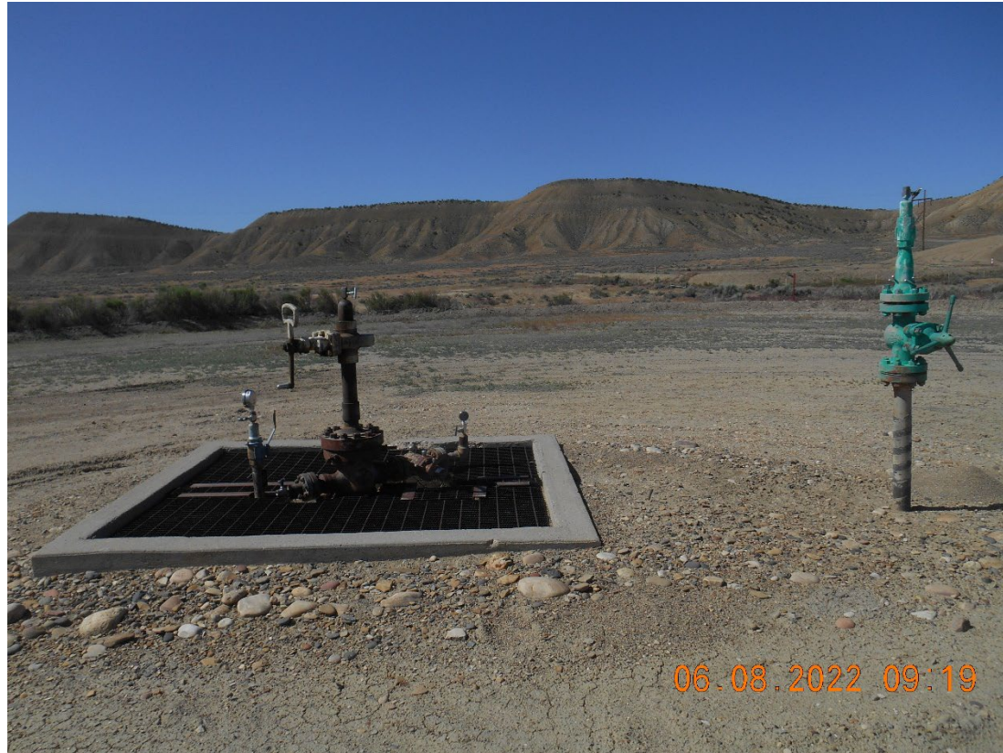
Injection wellhead. Temporarily Abandoned
