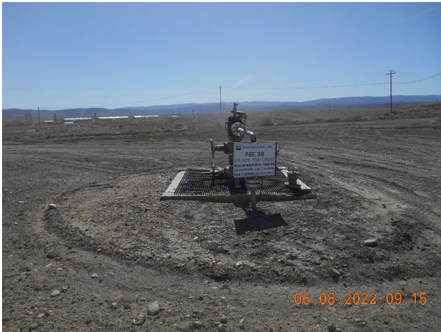
Injection wellhead.
