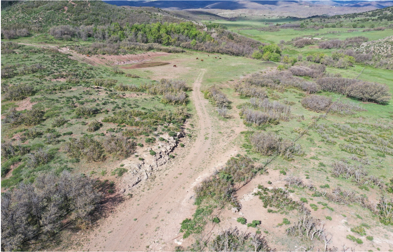
Photo 3. Drone aerial photo facing northwest along the access road. The access road has not been recontored and reclaimed.
