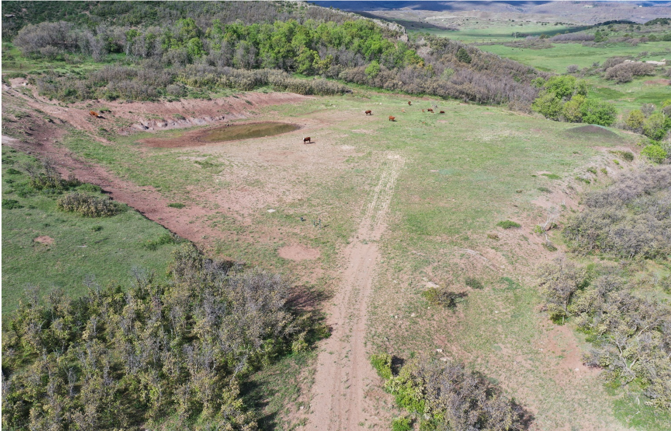
Photo 4. Drone aerial photo facing northwest shows the location has not been recontoured and reclaimed. The location disturbance is approximately 3.3 acres.
