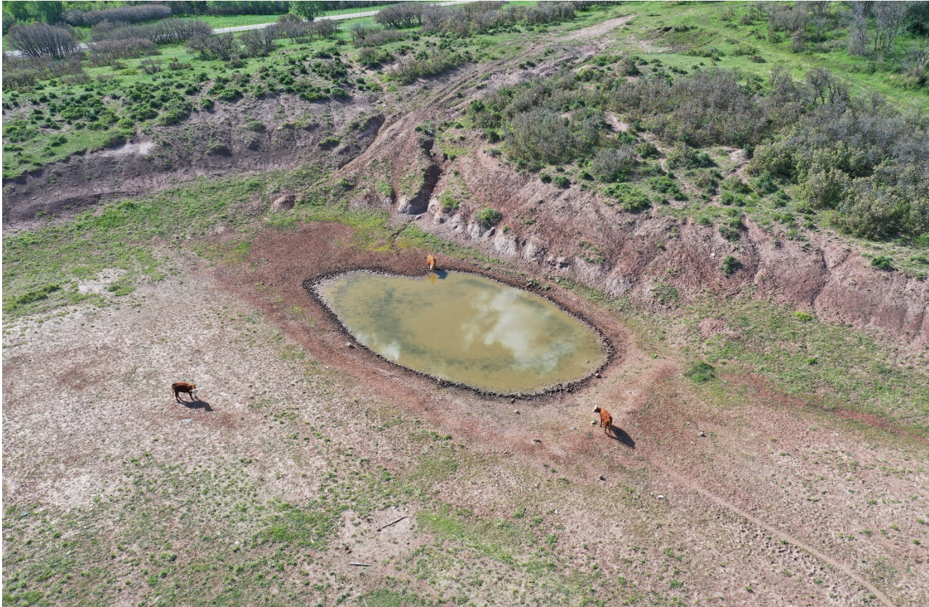
Photo 7. The pit was never backfilled and reclaimed. This photo shows the significant erosion along the cut slope.
