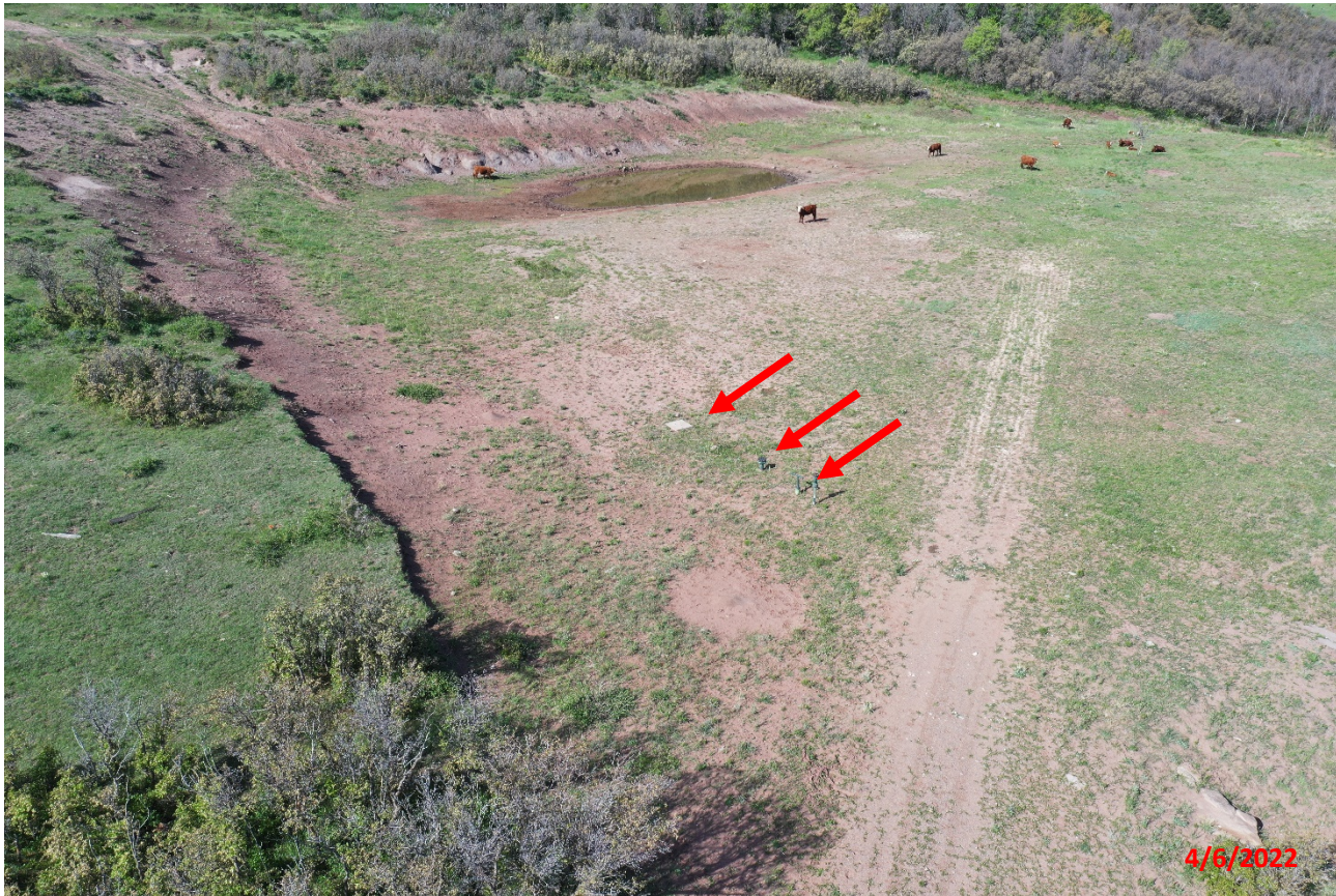
Photo 5. The pipeline risers still remain at the location shown at red arrows. Pipeline riser should have been abandoned per 1100 Rules.
