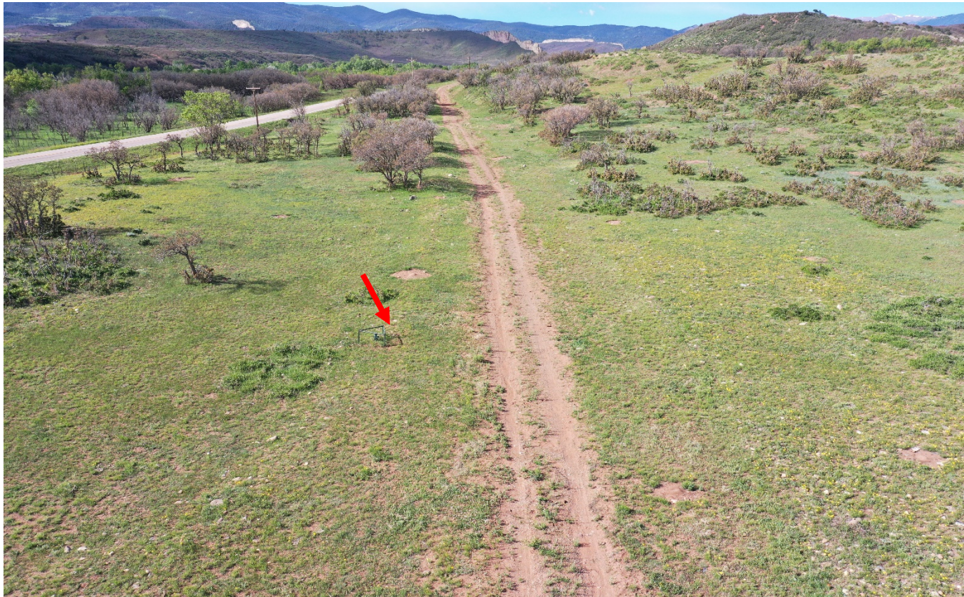
Photo 1. Drone aerial photo facing southwest along the access road. A pipe riser remains at the red arrow. The access road has not been reclaimed.
