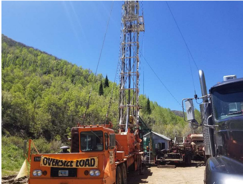
Photo 1. Workover on location replacing stuck pump.
