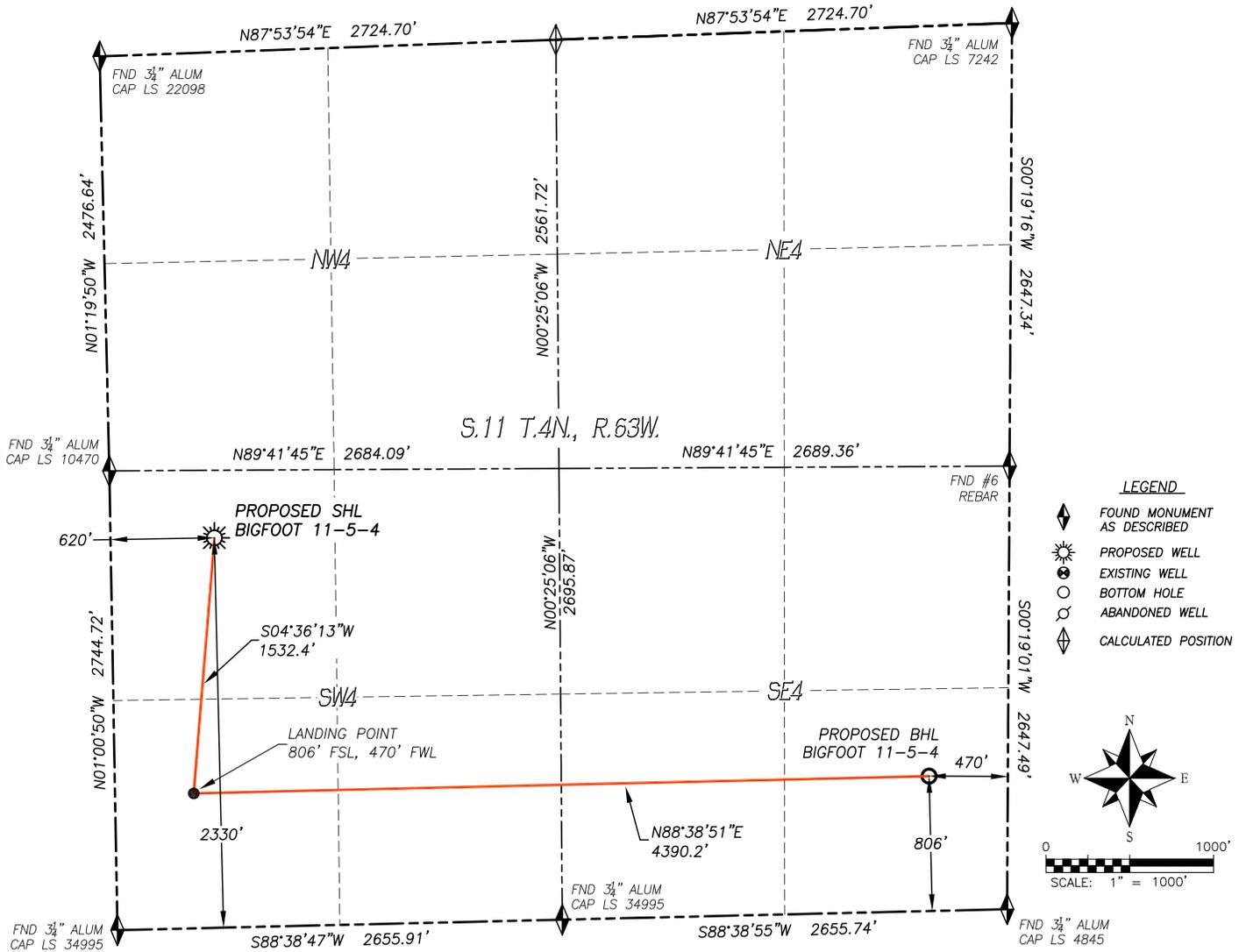
IN ACCORDANCE WITH A REQUEST FROM CONFLUENCE RESOURCES, DALEY LAND SURVEYING, INC. HAS DETERMINED THE SURFACE LOCATION OF THE BIGFOOT 11-5-4 WELL TO BE 2330' FSL, 620' FWL, AND THE BOTTOM HOLE LOCATION TO BE 806' FSL, 470' FEL, AS MEASURED AT NINETY (90) DEGREES FROM THE SECTION LINES OF SECTION 11, TOWNSHIP 4 NORTH, RANGE 63 WEST, OF THE 6TH PRINCIPAL MERIDIAN, WELD COUNTY, COLORADO.
