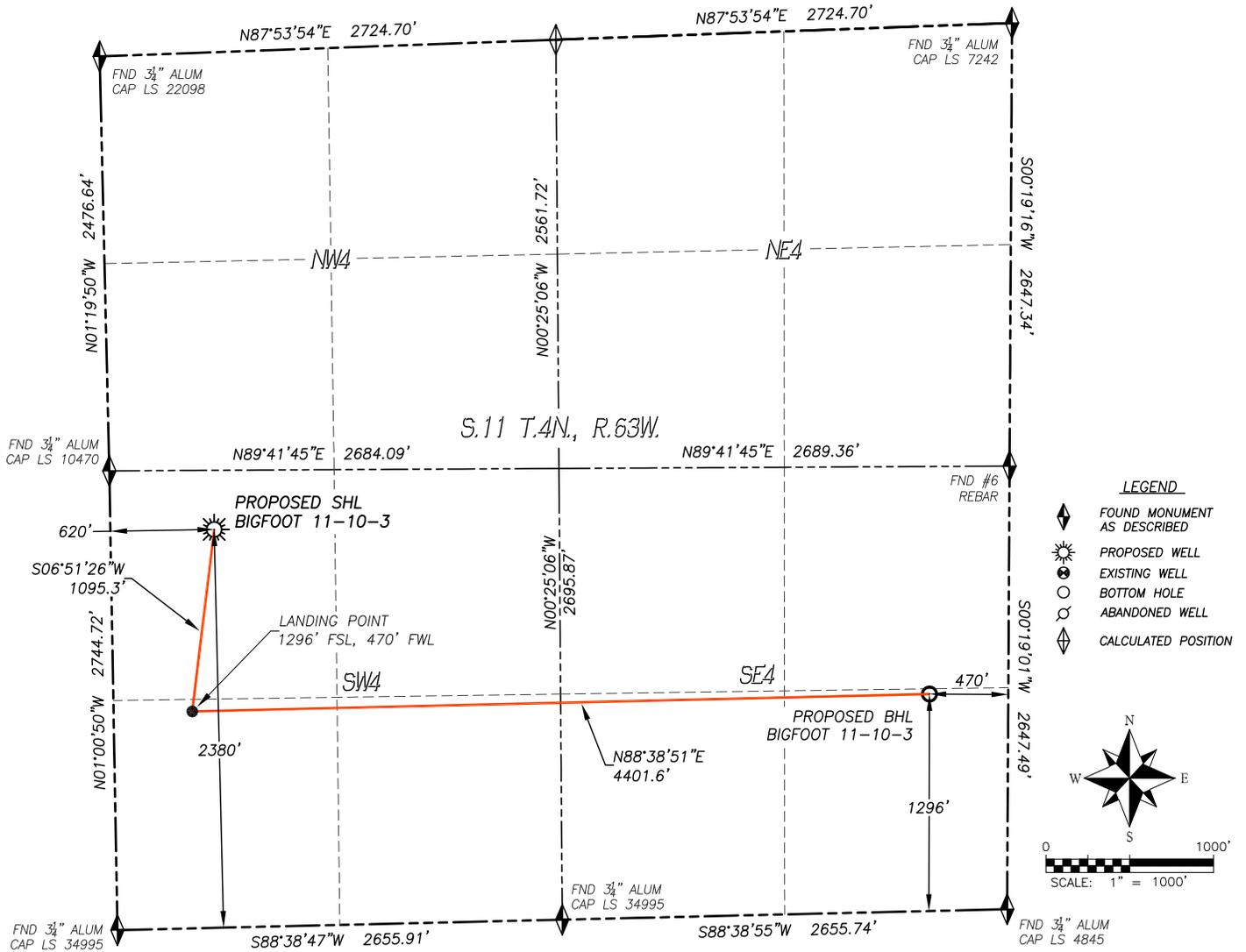
IN ACCORDANCE WITH A REQUEST FROM CONFLUENCE RESOURCES, DALEY LAND SURVEYING, INC. HAS DETERMINED THE SURFACE LOCATION OF THE BIGFOOT 11-10-3 WELL TO BE 2380' FSL, 620' FWL, AND THE BOTTOM HOLE LOCATION TO BE 1296' FSL, 470' FEL, AS MEASURED AT NINETY (90) DEGREES FROM THE SECTION LINES OF SECTION 11, TOWNSHIP 4 NORTH, RANGE 63 WEST, OF THE 6TH PRINCIPAL MERIDIAN, WELD COUNTY, COLORADO.
