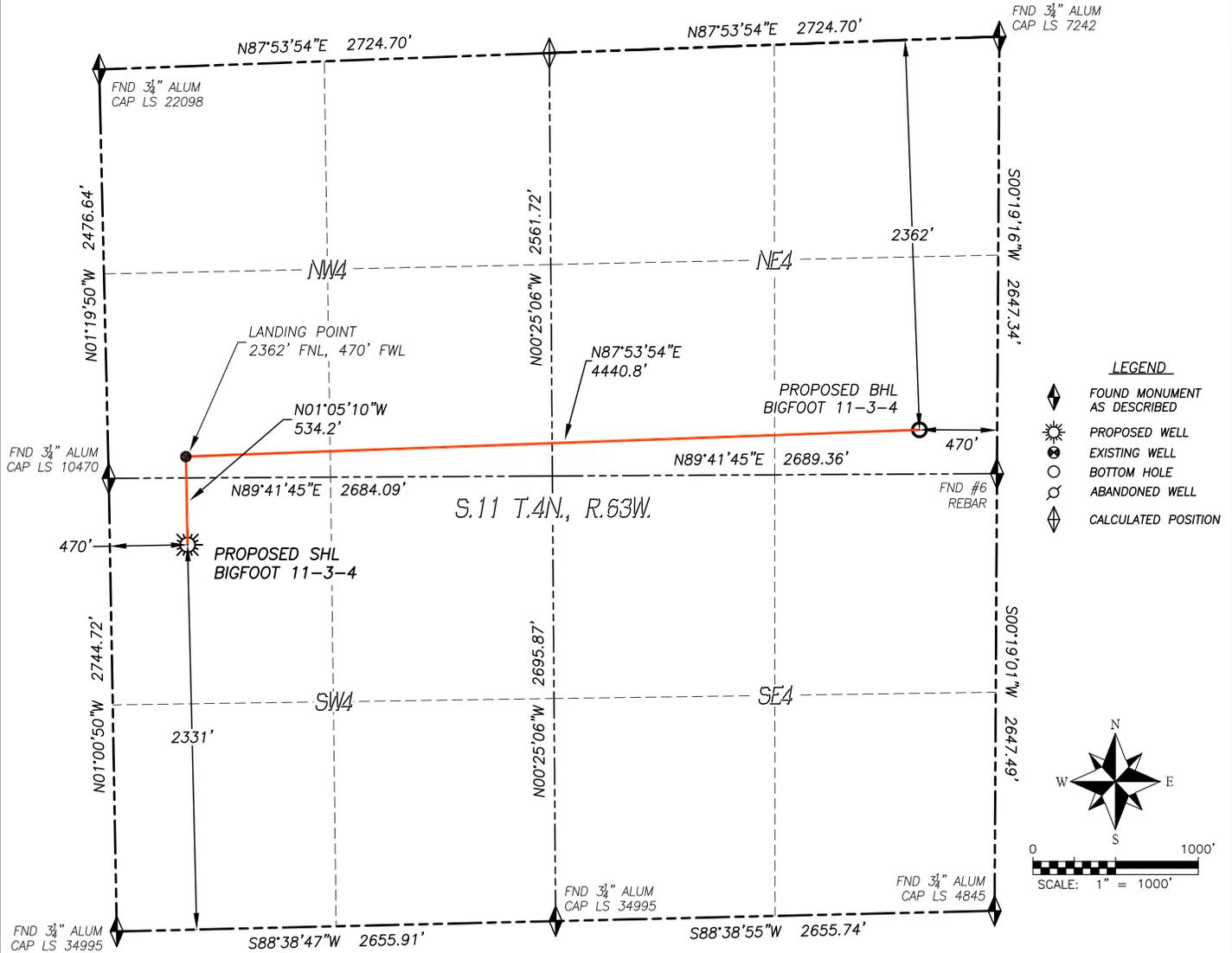
IN ACCORDANCE WITH A REQUEST FROM CONFLUENCE RESOURCES, DALEY LAND SURVEYING, INC. HAS DETERMINED THE SURFACE LOCATION OF THE BIGFOOT 11-3-4 WELL TO BE 2331' FSL, 470' FWL, AND THE BOTTOM HOLE LOCATION TO BE 2362' FNL, 470' FEL, AS MEASURED AT NINETY (90) DEGREES FROM THE SECTION LINES OF SECTION 11, TOWNSHIP 4 NORTH, RANGE 63 WEST, OF THE 6TH PRINCIPAL MERIDIAN, WELD COUNTY, COLORADO.
