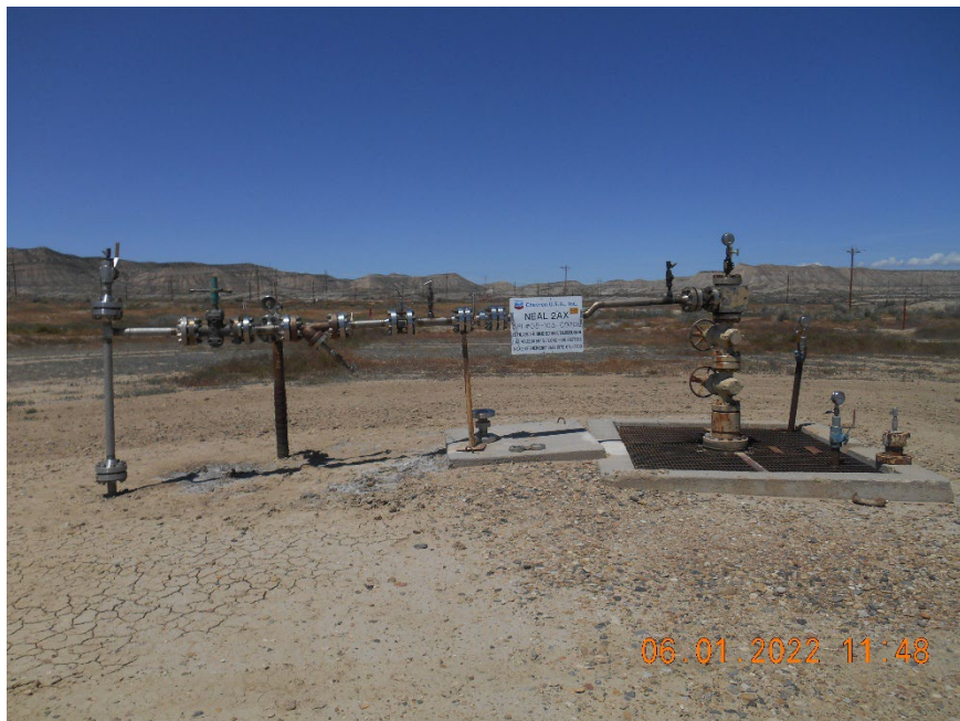
Injection wellhead
