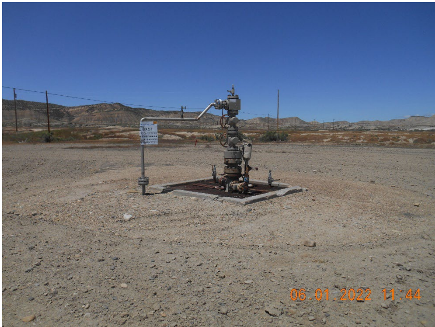
Injection wellhead
