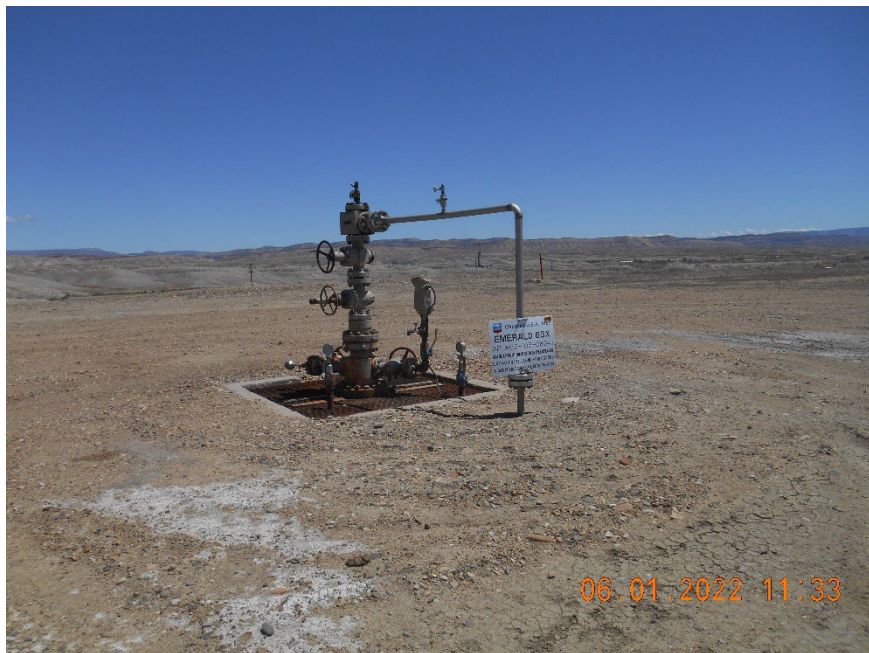
Injection wellhead
