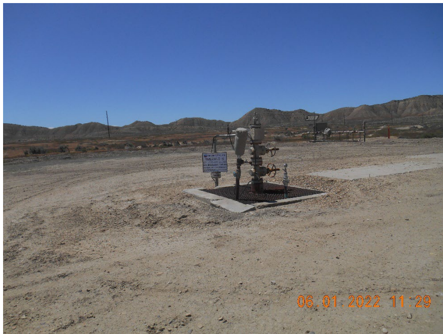
Injection wellhead
