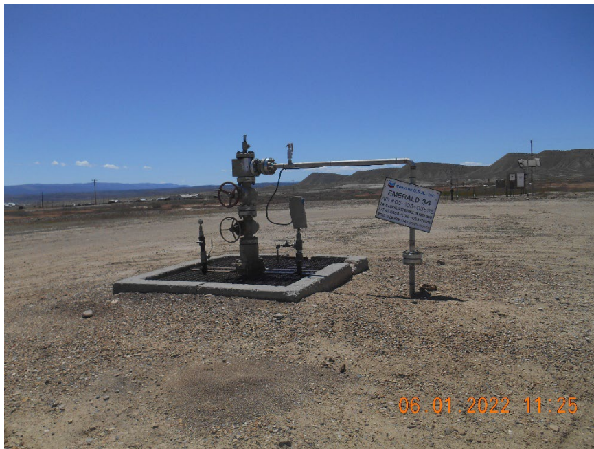
Injection wellhead
