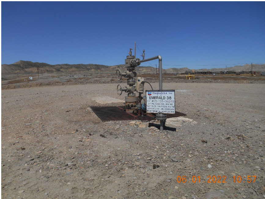
Injection wellhead.
