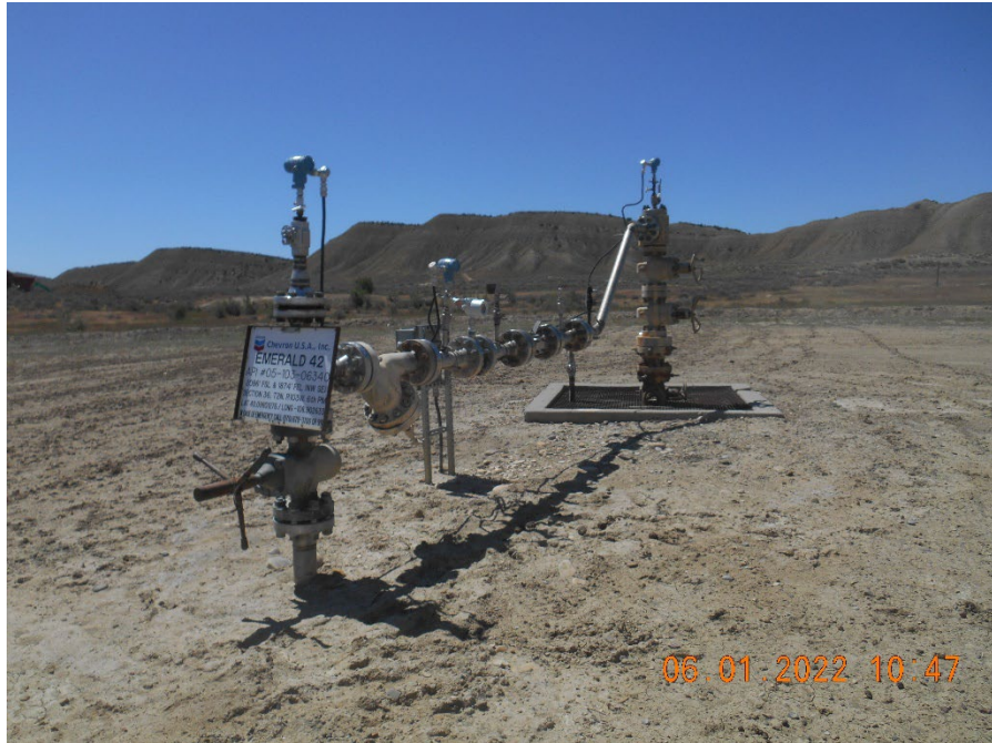
Injection wellhead. Water disposal well.
