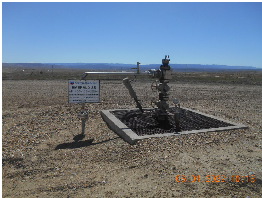
Injection wellhead
