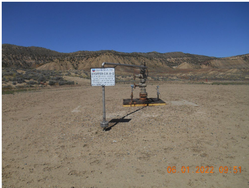
Injection wellhead
