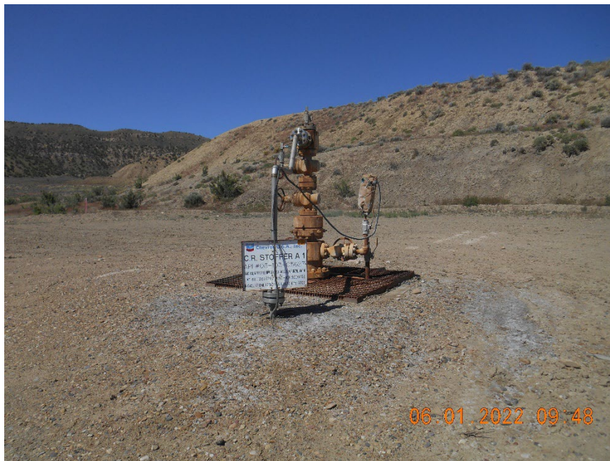
Injection wellhead
