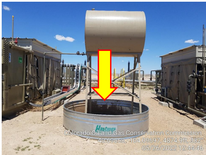
Photo 17 – Wildlife Netting is missing/disrepair
