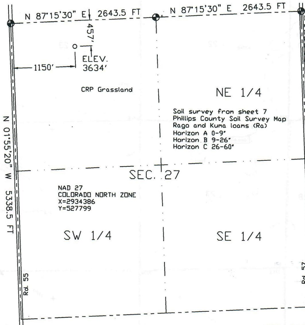
Basis of bearing is the north line of the NW 1/4 of Sec. 27, T9N, R43W of the 6th P.M., Phillips County, CO. bears N 87°15'30" E between set monuments
