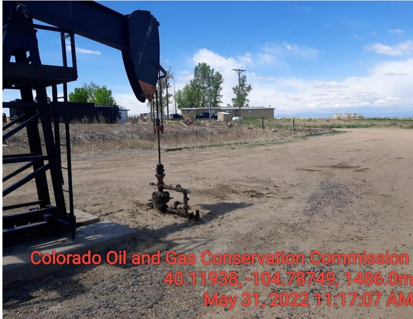
Photo 13 Road access shared with resident. Stained soil in front of well head
