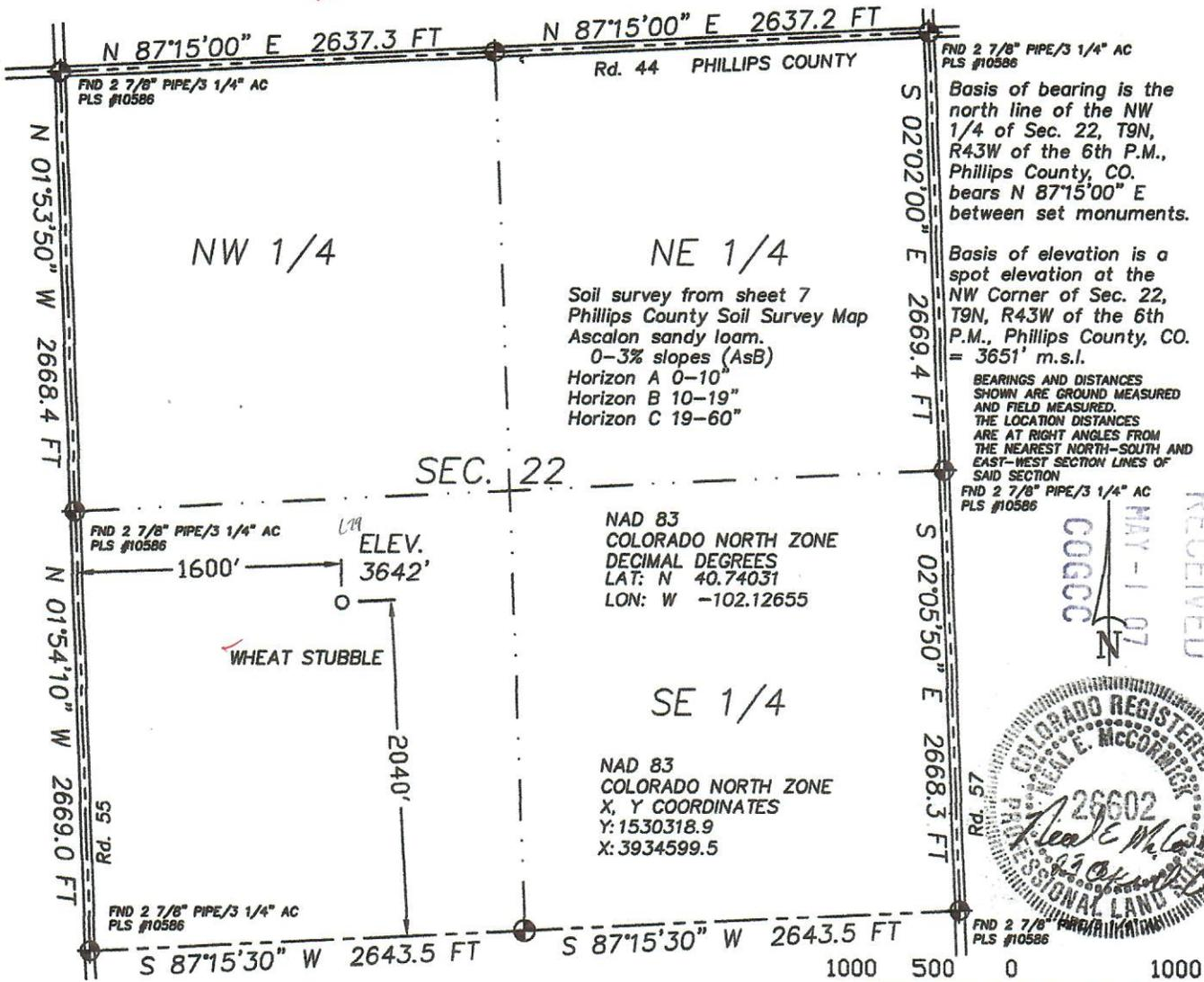
Basis of bearing is the north line of the NW 1/4 of Sec. 22, T9N, R43W of the 6th P.M., Phillips County, CO, bears N 87°15'00" E between set monuments.
