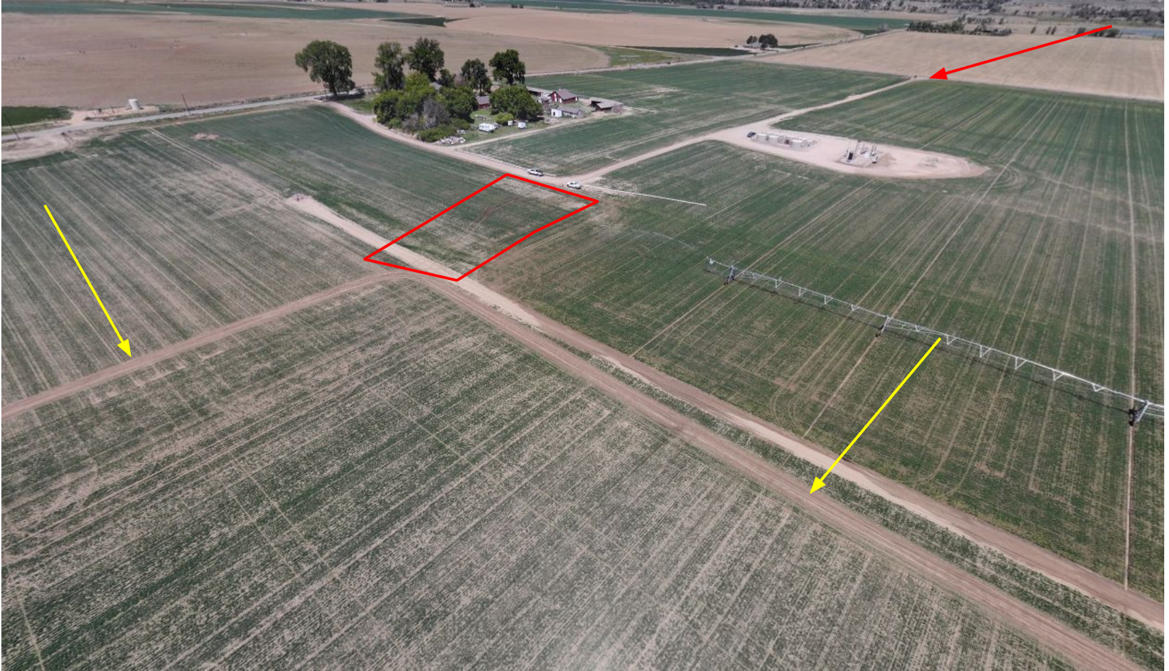
Photo 1. COGCC drone aerial imagery taken from location, facing Northwest. Photo illustrates the access point off CR 20.5 (red arrow) which is an established oil and gas access road for the Crestone Peak Williams Unit facility. The red box is the approximate access road that will be constructed for the well pad. The yellow arrows illustrate the perimeter ditch and berm BMP that is being installed around the entire perimeter of location.
