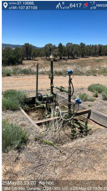
IMG 13 Wellhead with encroaching weeds
