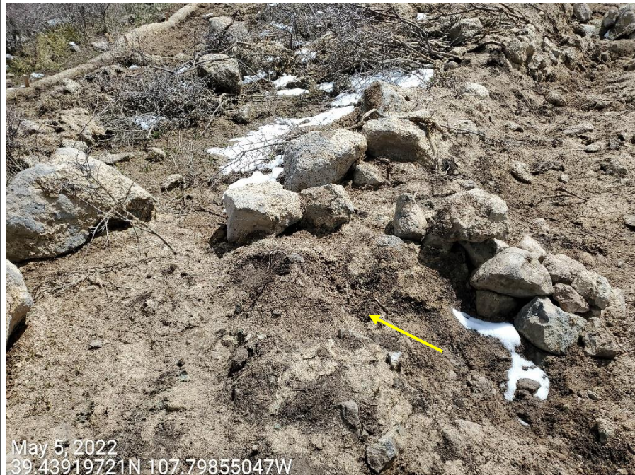
Photo 12: Continued from photo 11. Photo example showing low points within the ditch along the north end of the Location, where stormwater is discharging from, rather than flowing into the northwestern sediment traps.
