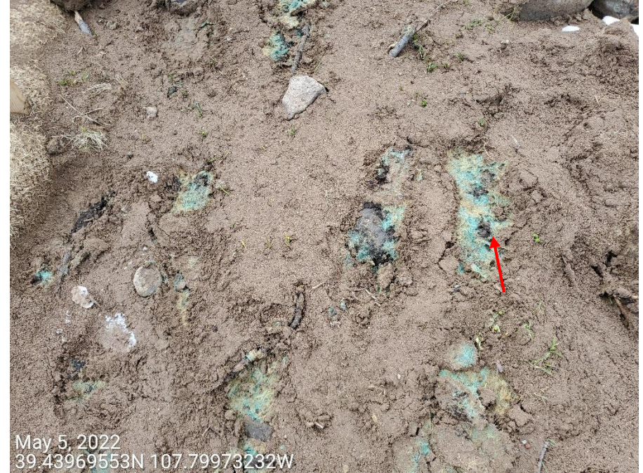
Photo 9: Photos example shows sediment deposition as a result of the erosion degradation from the unstabilized fill slopes. Photo right also shows remnants of the hydromulch that was previously applied, and is now covered with sediment from the fill slopes.
