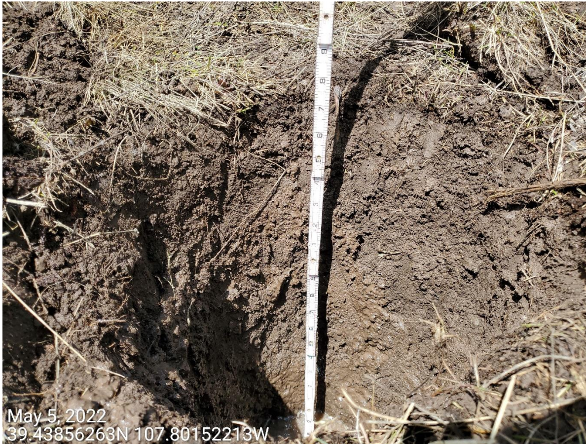
Photo 17: Photo example of one of the topsoil test pit conducted within the adjacent reference area. Topsoil on Location could have exceeded 22 inches in depth. Operator topsoil plan stated 4,700 cy of material would be salvaged; actual amount salvaged by Operator was 2,300 cy.
