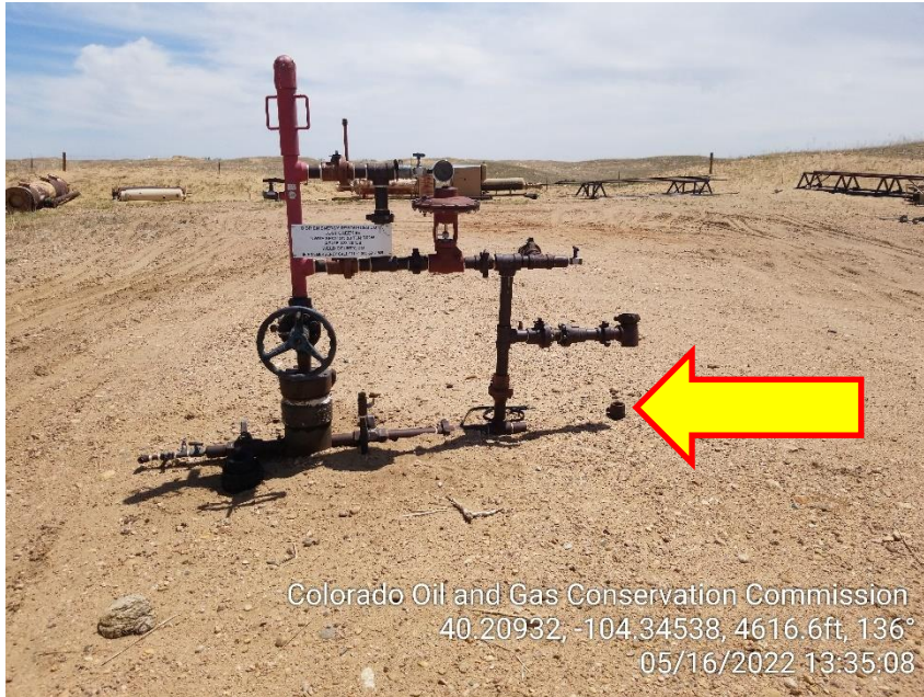
Photo 1 – Wellhead – Unmarked Riser
