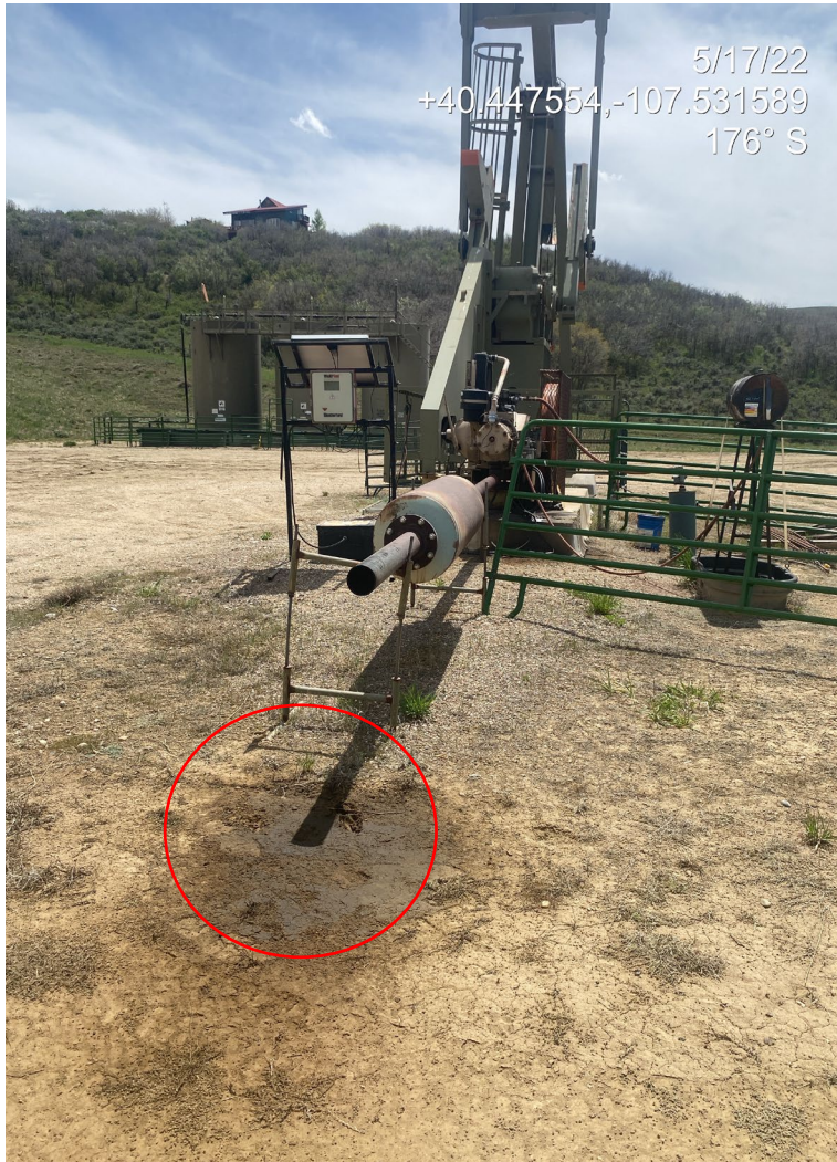
Photo 3. Photo taken from the pipe to the north of the pump jack shows stained soils below the outlet.
