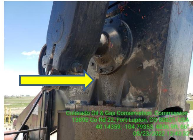
Photo 7 Stained concrete due to leaking seal.
