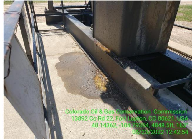
Photo 5 Pump Jack seal is leaking.
