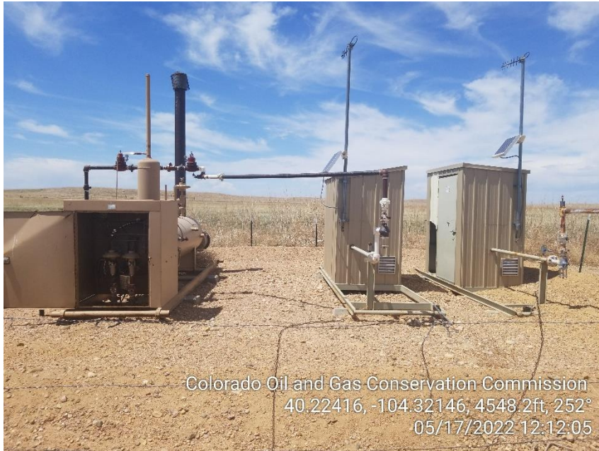
Photo 13 – Separator and Gas Meters
