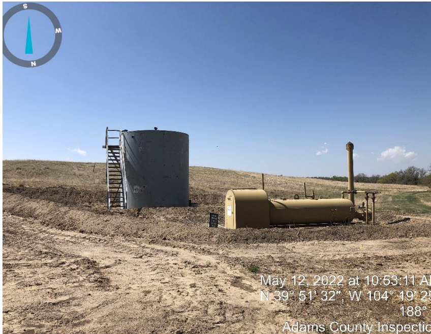
Photo #1 Crude tank and separator.
