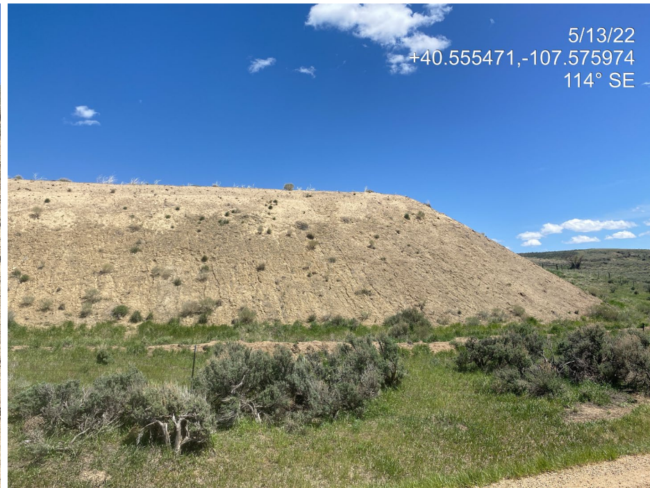
Photo 10. Photo taken from the west of the Location shows rill erosion occurring on the bare, unprotected fill slope.
