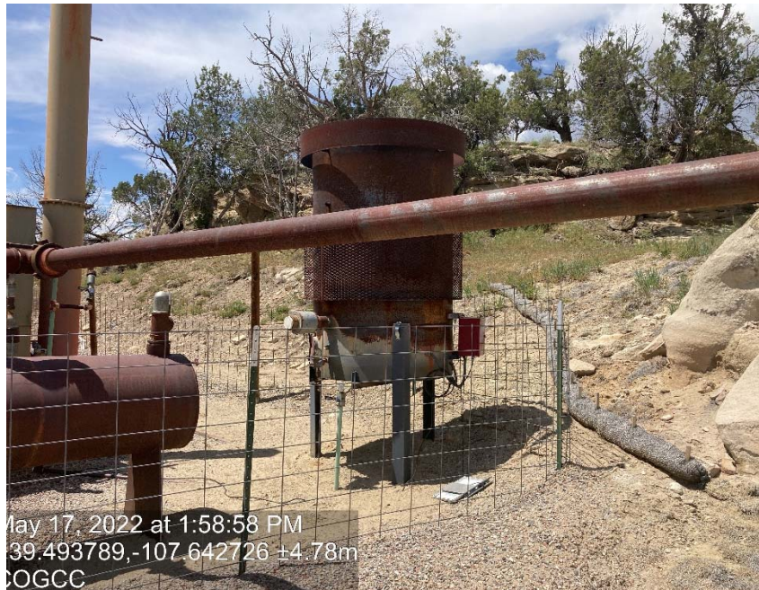
Stored equipment (ECD is disconnected from tanks and gas)
