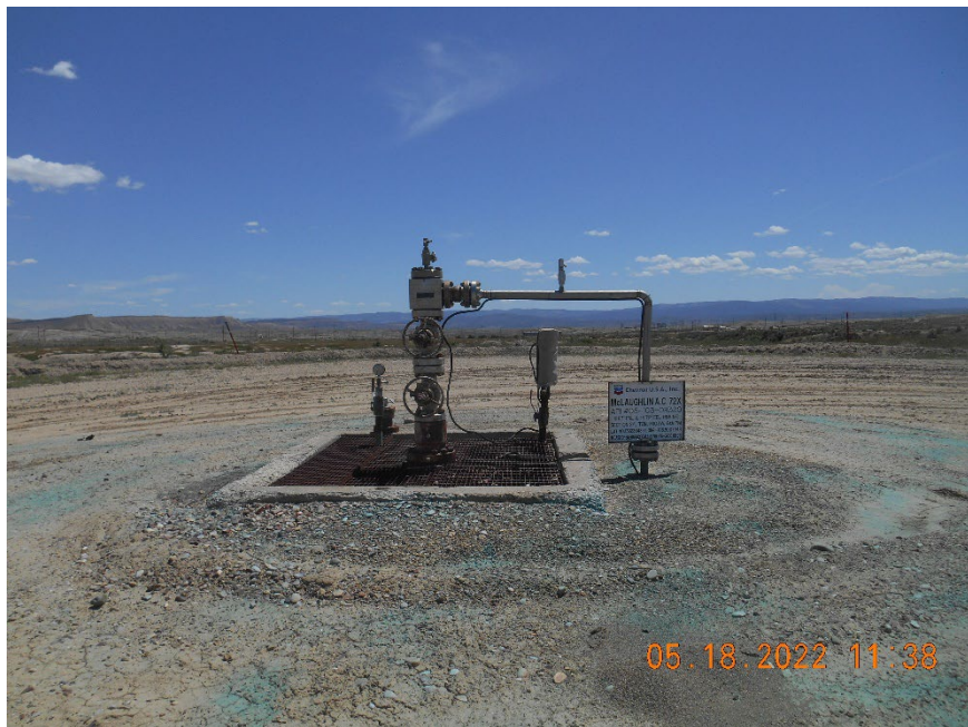
Injection wellhead.
