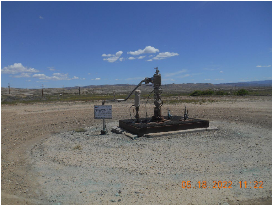
Injection wellhead.
