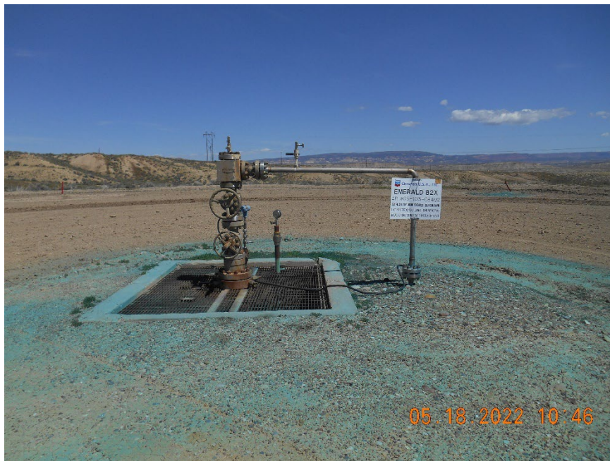
Injection wellhead
