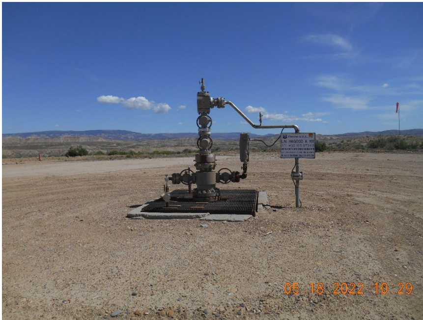
Injection wellhead
