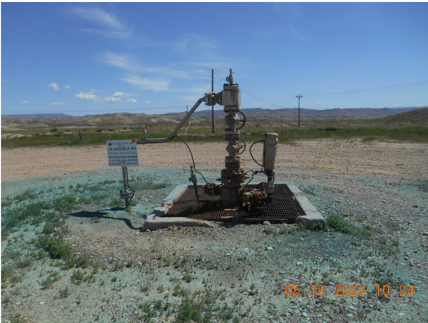
Injection wellhead
