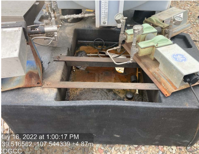
Chemical containment full of fluid and unused pumps
