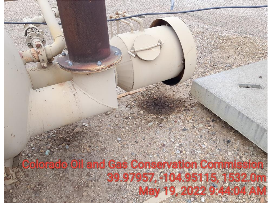
Photo 4 Stained soil and mechanical issue Hoz heated separator
