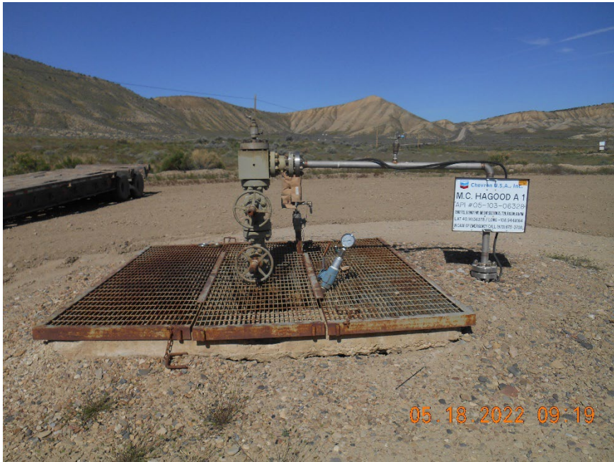
Injection wellhead
