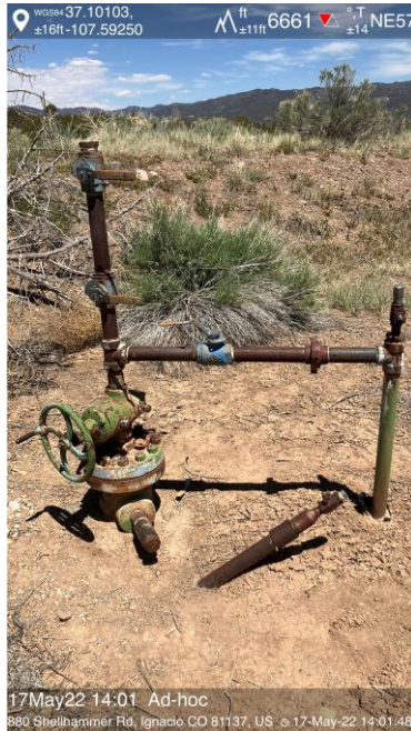
IMG 03 Wellhead with accessible bradenhead
