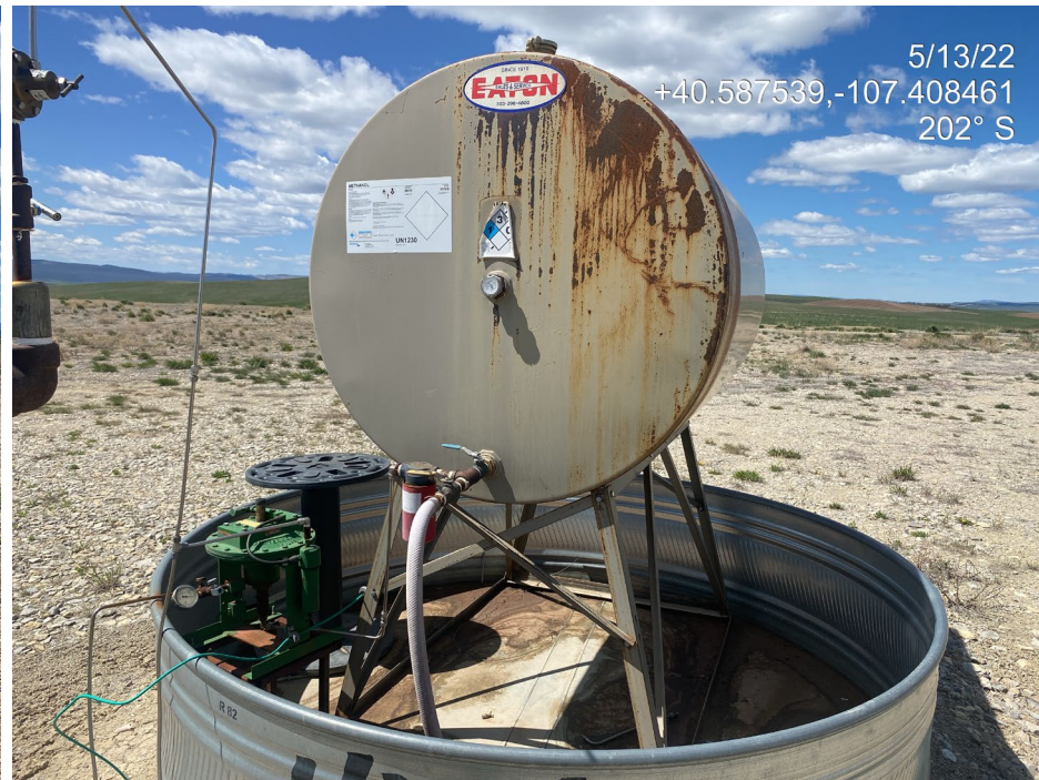
Photo 6. Photo taken from the north of the Location adjacent to the compressor shed shows a methanol tank secondary containment stock tank lacking wildlife protection BMPs.
