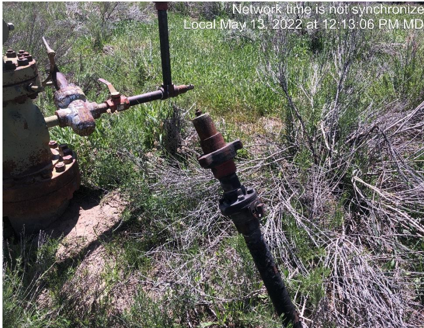
Photo #6718 Flowline improperly abandon.
