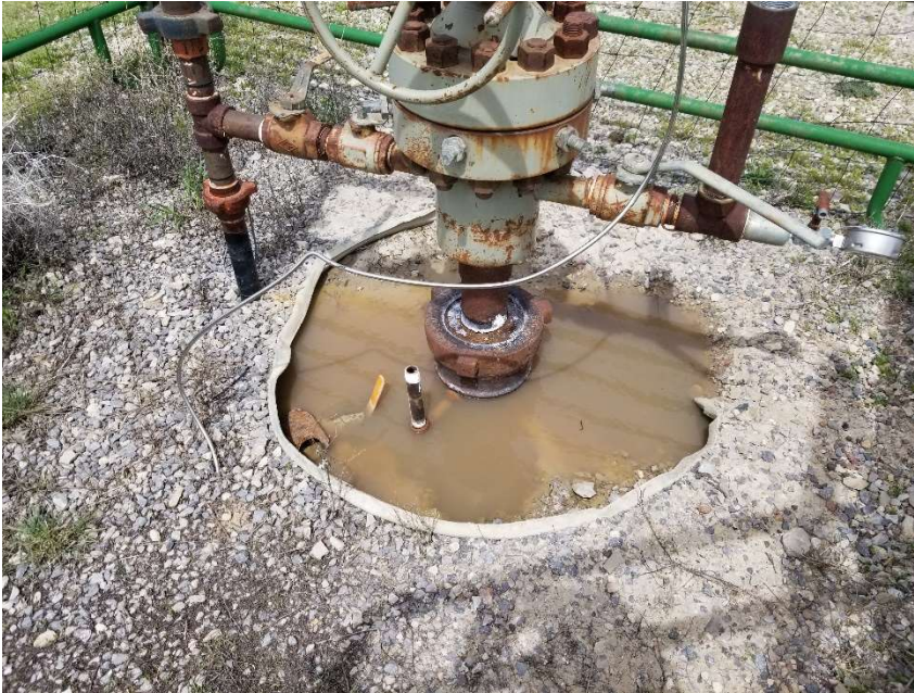
Photo 2. Bradenhead access has been installed. Water present in cellar.
