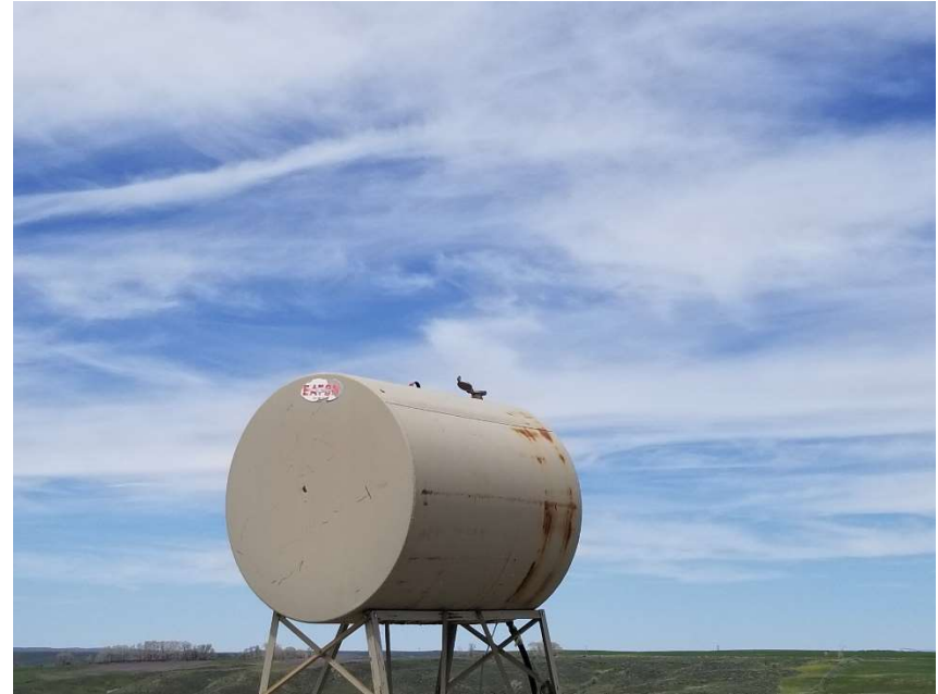
Photo 5. Gauge hatch open on diesel fuel tank.
