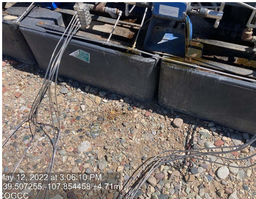
Pump leaking
