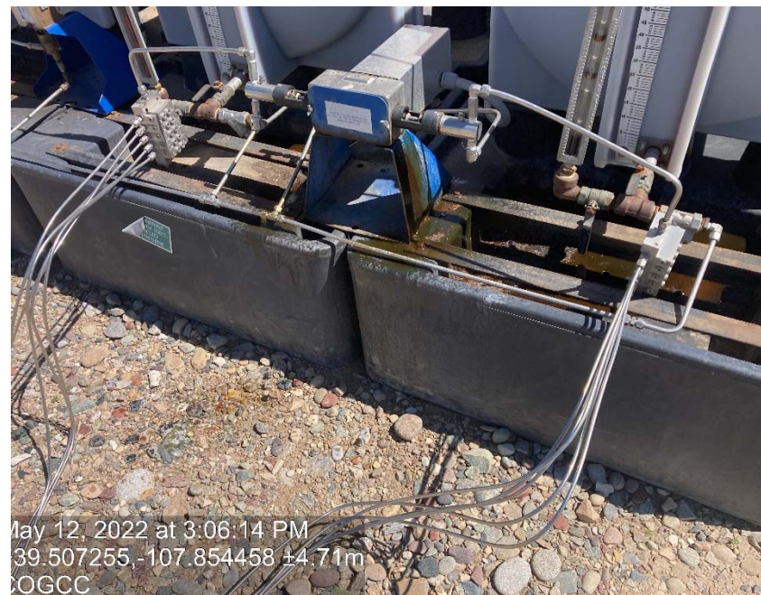
Pump leaking
