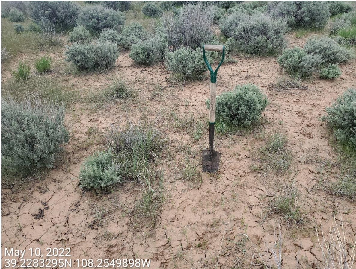
Photo 6: Photo taken from the adjacent reference area, to compare to the observed compaction concerns on Location. Photo shows reclamation specialist was able to easily penetrate approximately 10 inches of soil on the reference.
