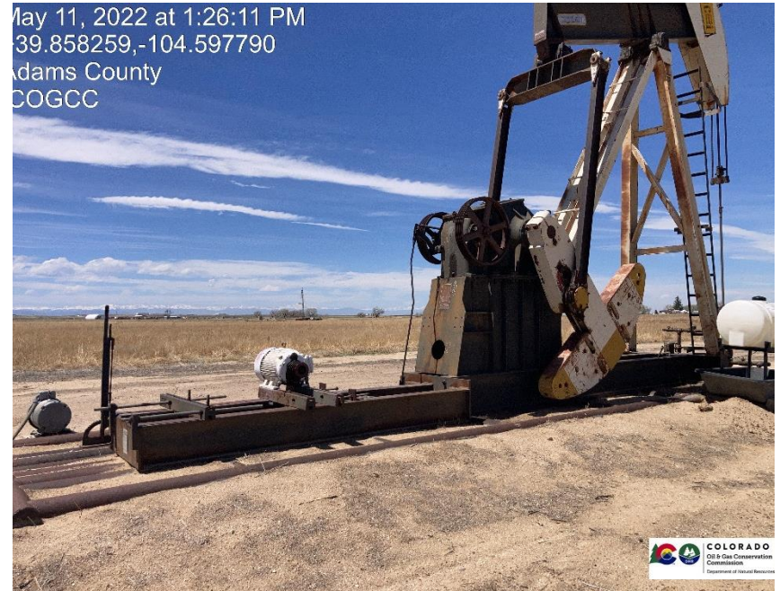
Pic 2 pumpjack motor does not have belt connected to pump jack counter weights
