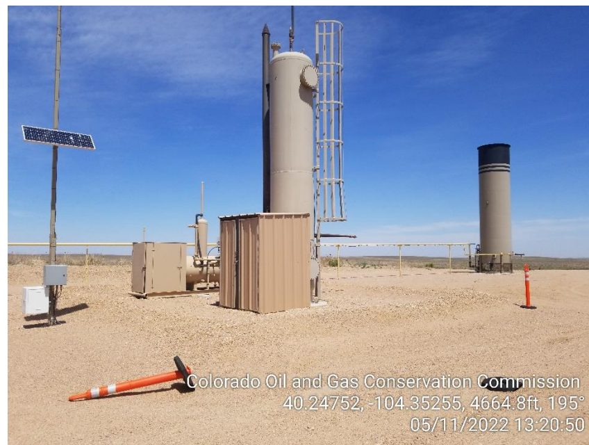
Photo 6 – Separator, Heater Treater and ECD
